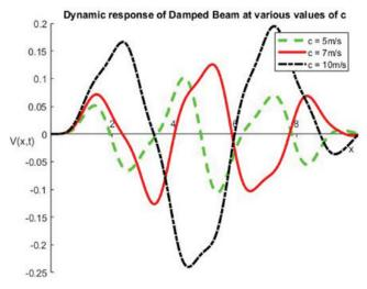
Figure (1.2): Dynamic response of damped beam at various values of c
