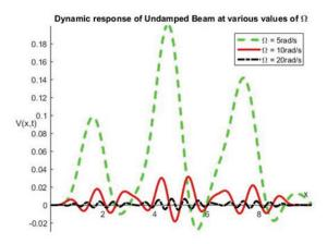
Figure (1.1): Dynamic response of undamped beam at various values of  $\Omega$
