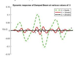
Figure (1.0): Dynamic response of damped beam at various values of  $\Omega$
